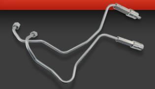
Common rail diesel fuel systems operate on extremely high pressure. These systems typically have an operating pressure above 2000 bar (29000 PSI).
